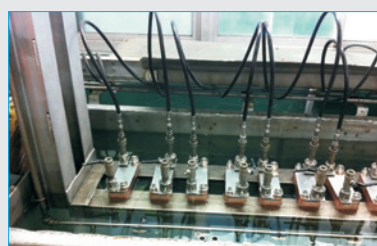
Pressure Leakage Test
